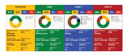
apps to view equipment status and alarms in real-time. Receive Microsoft Teams, text messages and email notifications based on configurable events such as the machine running with the feedrate override turned down. Take your shop floor to the next level using Scytec DataXchange.
